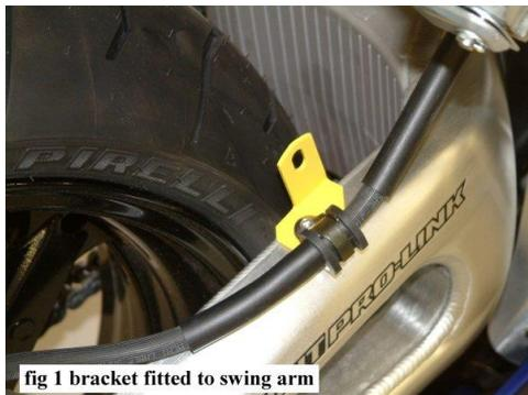
fig 1 bracket fitted to swing arm
